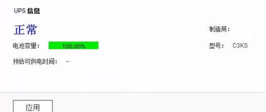
The screenshot shows the 'UPS 信息' (UPS Information) page. The status is '正常' (Normal) in large blue characters. Below it, '电池容量:' (Battery Capacity) is shown as a green bar at '100.00%'. '预估可供电时间:' (Estimated Runtime) is shown as '--'. On the right side, '制造商:' (Manufacturer) and '型号:' (Model) are listed as 'C3KS'. At the bottom, there is an '应用' (Apply) button.
